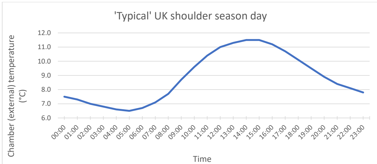
Figure 1 - Chamber temperature profile for a 'typical' UK shoulder season day.
