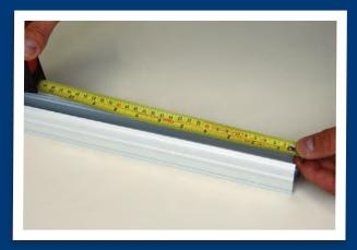
**1.** Measure and mark off the headrail deducting  $15\,\mathrm{mm}$  from your finished blind siz . This is to take into account the length of gear housing.
