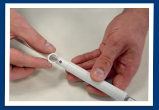
**4.** Once they are aligned, take one of the clips and insert through the hole attaching the crank arm to the aluminium rod.
