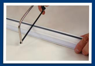
**2.** Cut the headrail to your required width and file to make sure there are no sharp edges, then cut your axle rod 17mm less than the headrail.
