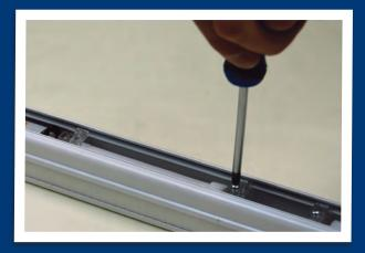
**6.** Firmly tighten the bridge screw on each spool to hold in place.
