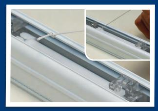
**7.** Take your cord and tie a knot in one end (fig 1) then attach to one of the grooves on the barrel of the spool and pull tight ensuring it's securely held in place (fig 2)
