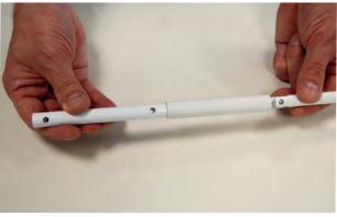
3. Test fit by inserting the crank arm into the rod to ensure the holes line u . Repeat with the hook.
