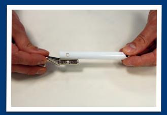
1. Once you have cut your aluminium rod to the required length, you will need to line the hook up with one end of the rod and mark the position of the hole on the rod. The hole on the hook should line up with the mark on the aluminium rod. Take your drill and drill a hole all the way through the rod.
