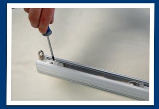
**5.** To secure the gear housing to the headrail ensure both screws have been loosened off on the bridge so it slides into the channel inside the headrail. Push completely in then tighten up both screws on the bridge to secure in place.
