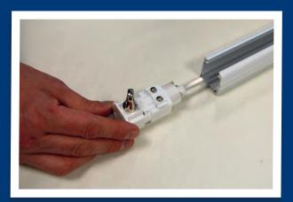
**3.** Slide each spool inside the headrail ensuring the cord guides always face towards the outside. Insert the axle rod through all the spools inside the headrail and connect the axle rod to the gear housing. Finally tighten the screw with a Phillips screwdriver.
