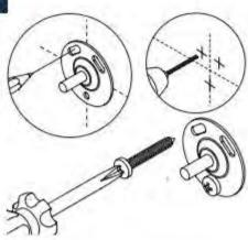
On your horizontal line mark the bracket positions using the back plate as a guide. Drill the holes and secure the back plate with the appropriate fixings.
