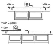
Measure the poles as shown above. If you have two poles, repeat the measurement on both sides of the window. Poles can be cut down to shorten their length. Both poles should be of equal length so that they meet in the centre.
