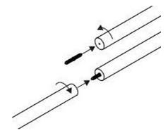
If joining 2 poles together, use the joining screw provided. The poles must be joined in the centre and supported by the centre bracket.
