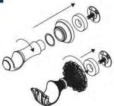
Assemble the brackets onto the back plates and secure by turning the bracket body clockwise until it is tight. Ensure that the cup is upright on completion of tightening. 4
