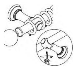
Place the pole on the brackes with the last ring on each side between the finial and end bracket. Finish by tightening the screws to ensure your pole is secure.
