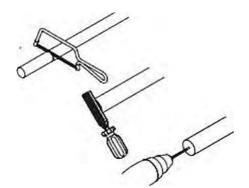
If cutting down, when you are certain your measurements are correct, mark the pole and cut. Wrap masking tape around the pole to avoid damage. File any sharp edges and drill a small hole in the centre of the pole.
