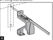
. Position the brackets on the wall and mark the holes on the wall, Fig. 4.
