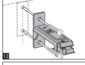
4. Using the correct screws fix the brackets securely, Fig. 12. Alternative wall fixings should be used where necessary.
