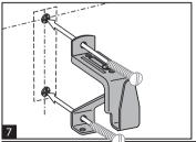
4. Using the correct screws fix the brackets securely, Fig. 7.
