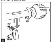
1. Extend pole to the approximate required length, slide one curtain ring to each end of the pole (next to finials) and place pole onto the wall brackets. At each end of the pole there is a small hole on the underside. These holes locate on the protruding lugs in each end bracket arm (Fig. 8).
