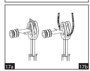
2. Extend the neck of the pulley and secure in higher position using a pin or small nail. Remove the central barrel of the pulley by pulling it down and then out (Fig. 17a). Place the cord inside the pulley and replace the barrel ensuring it clicks into place (Fig. 17b).
