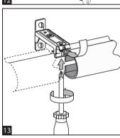
5. Attach supports by hanging the clip in the channel of the pole. The bracket is extendable by loosening the small screw underneath and sliding the bracket forwards or backwards.
