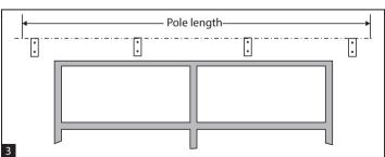
The pole is adjusted in length by sliding the inner pole into or out of the outer pole.
