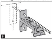
1. Place the pole on the outer brackets and position the intermediate bracket and mark the holes on the wall, Fig. 9.
