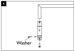
Using the screw provided secure the arm of the dormer rod into the bracket. Do not over tighten the screw as this will limit movement of the dormer rod. (fig 5)
