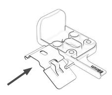
For top fix, the above image shows how the bracket is attached.
