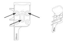
For face fix within a recess, the above image shows which locators to use on the fitting tool.
