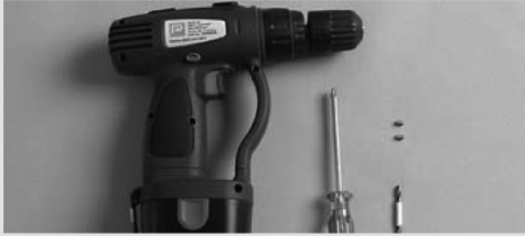
A1. Fitting tools required include Ø4mm drill bit, star point screwdriver.
