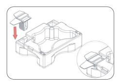
1. Place the top corner bracket into the slot on the fitting tool.
