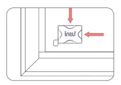
4. Position bracket behind the rubber bead and carefully push until the metal legs are behind the rubber bead.
