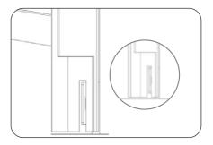
8. Push the slot at the base of the extrusion over the bottom corner bracket. Gently push the extrusion against the glass to ensure tape has adhered. Repeat for both sides.
