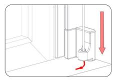
12. If your blind requires further tension, pul the cord through the bottom button until you feel the blind has sufficient tension and tie a fresh knot.
