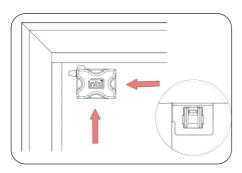
Position bracket behind the rubber bead and carefully push until the metal legs are behind the rubber bead.
