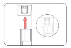
6. Slide the side extrusion up until its slots into the top corner fixing bracket. The side extrusion should rest under the bracket.
