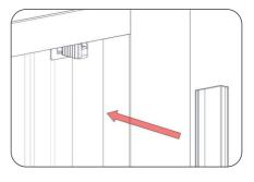
5. Ensure the glass is clean and free from debris by cleaning it with glass cleaner. Place the flat side of the side extrusion against the glass with the notch to the bottom.
