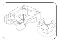
3. Place the bottom corner bracket into the slot on the fitting tool.
