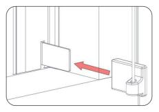
10. Align bottom button with bottom corner brackets. Slide the bottom button onto the bracket until it locates. Repeat both sides.
