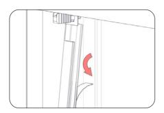
7. Pivot the extrusion towards yourself so you have access to the back. Peel the backing from the glass tape and slowly place the extrusion against the glass.
