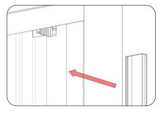
5. Place the flat side of the side extrusion against the glass with the notch to the bottom.
