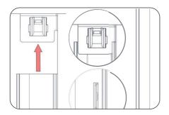
6. Slide the side extrusion up until its slots into the top corner fixing bracket. The side extrusion should rest under the bracket. Push the slot at the base of the extrusion over the bottom corner bracket. Repeat for both sides.
