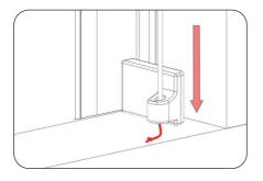
11. If your blind requires further tension, pull the cord through the hole in the bottom button until you feel the blind has sufficient tension and tue a fresh knot.
