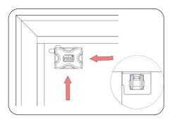
2. Position bracket behind the rubber bead and carefully push until the metal legs are behind the rubber bead. Check bracket is square to the sides of the bead and is secure. Repeat for other side.
