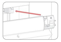
8. Align headrail endcaps with top corner fixing brackets and push fully home.
