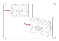
7. At the appropriate position(s) on each side profile, fit retention clips (long side profiles only). Press into position using the fiting tool.
