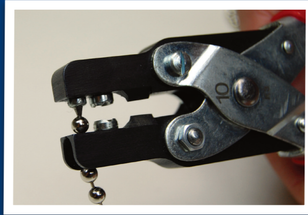
11. Remove the chain from the pliers and place the opposite end in and firmly press down until this splits completely in half and falls away from the chain.
