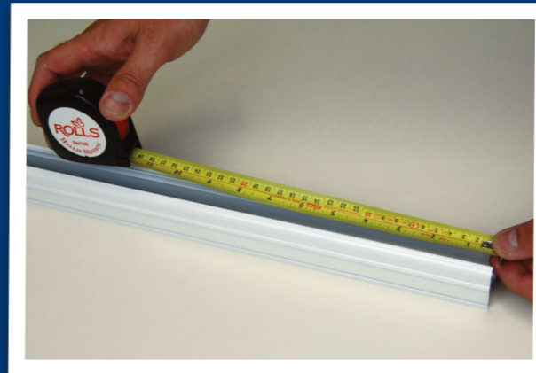
1. Measure and mark off the headrail deducting 15mm from your finished blind size, this is to take into account the length of gear housing.
