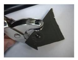
Squeeze the pliers to close the eyelet.
