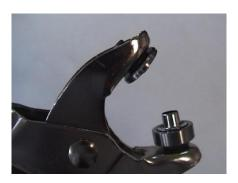
Place the hole in the material over the eyelet barrel.
