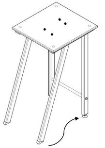
Use the 2 rear adjustable feet to level the bench.
