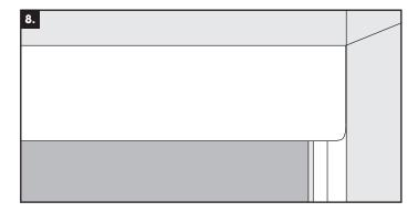
**Step 8.** Fit the fascia to the lipped metal plate ensuring you don't move its position on the bracket whilst making sure its fitted flush inside the recess, this will ensure the Cov-A-Blind bracket cannot move once positioned correctly.
