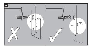
**Step 6.** Before fitting the fascia ensure the lip on the metal Cov-A-Blind plate has hooked onto the magnetci disc on the bracket.
