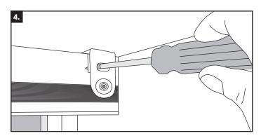
**Step 4.** Tigthen the M4 screw so that the end sits flush with the front of your headrail. Repeat this process for all other brackets.
