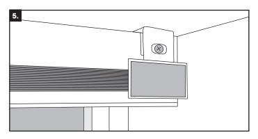
**Step 5.** Attach the Cov-A-Blind lipped metal plate to the magnet on the bracket ensuring the lip hooks securely onto the round magnetic plate.
